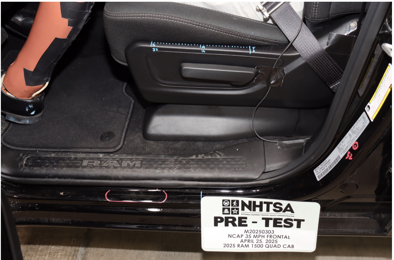
Photo No. 036 - Pre-Test Driver's Seat Fore-Aft Markings
