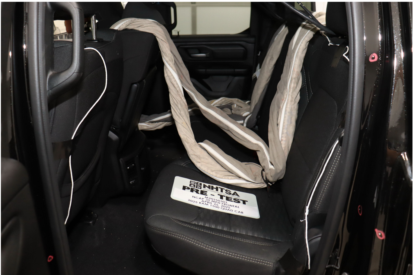
Photo No. 028 - Pre-Test Dummy Cable Routing
