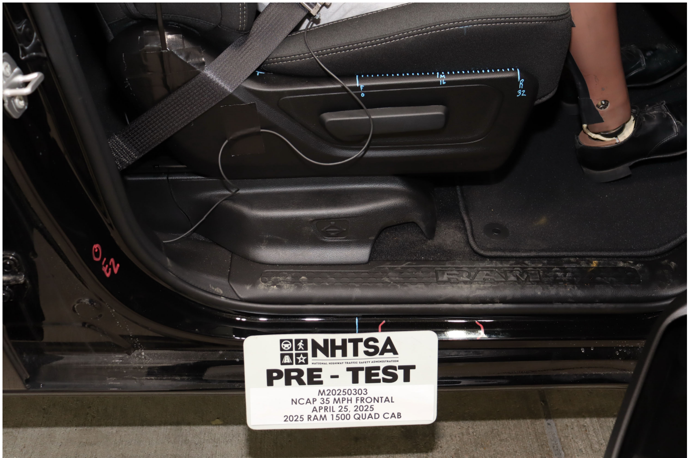
Photo No. 059 - Pre-Test Passenger's Seat Fore-Aft Markings
