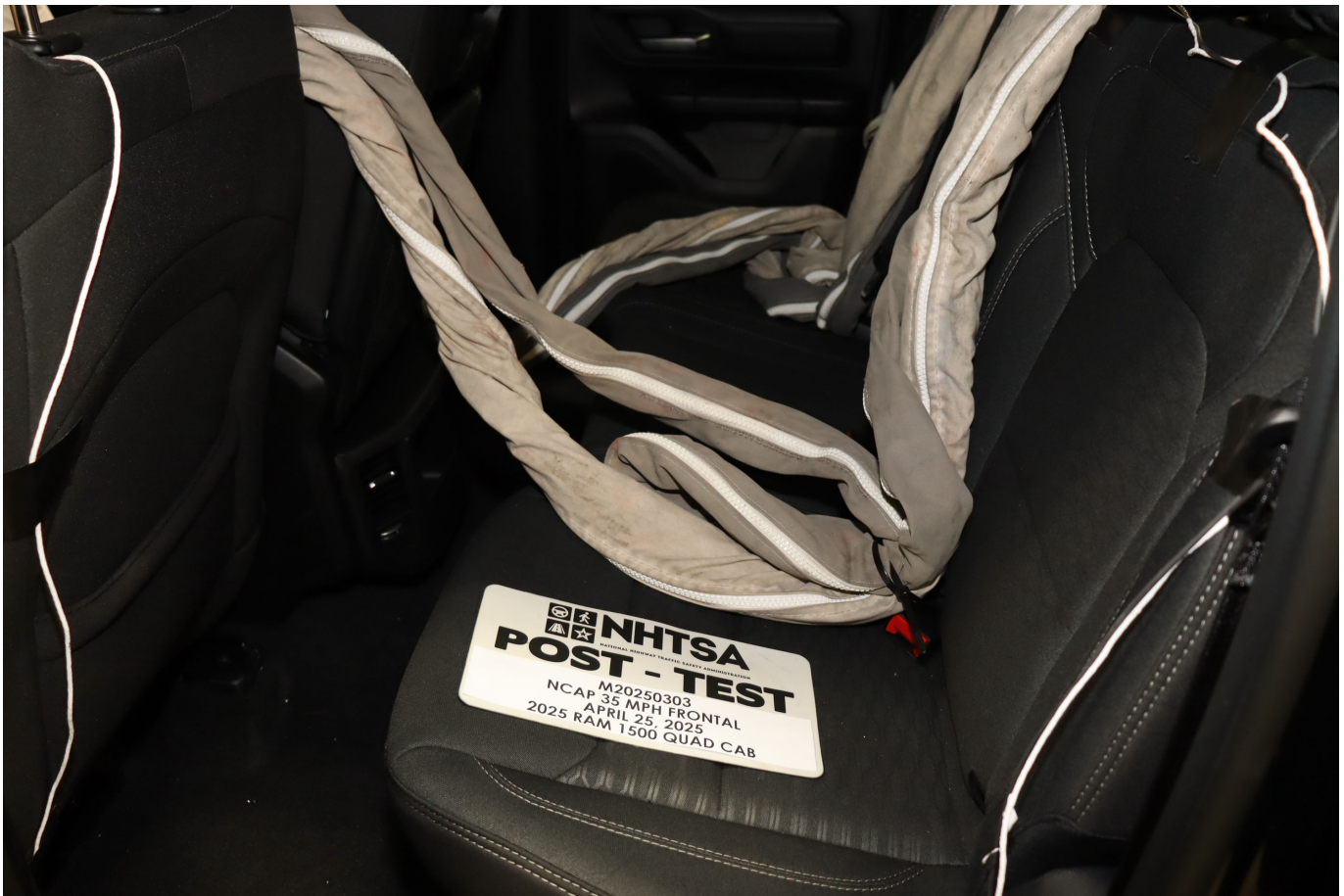
Photo No. 029 - Post-Test Dummy Cable Routing
