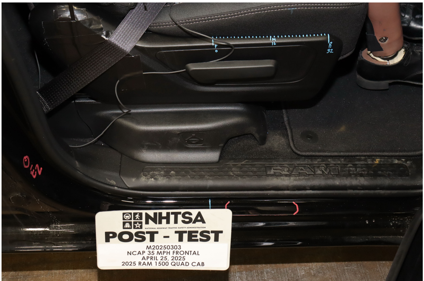
Photo No. 060 - Post-Test Passenger's Seat Fore-Aft Markings
