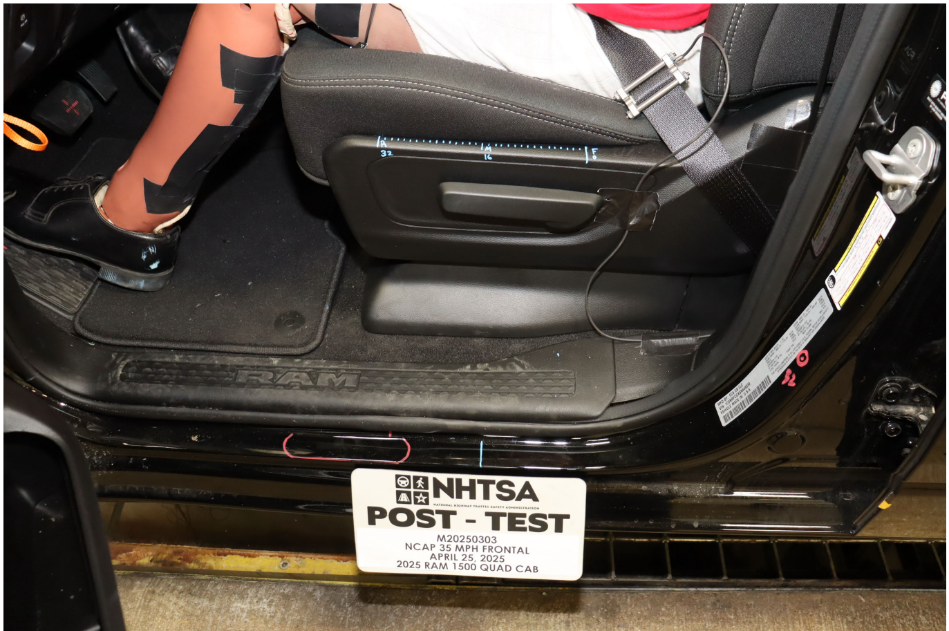
Photo No. 037 - Post-Test Driver's Seat Fore-Aft Markings
