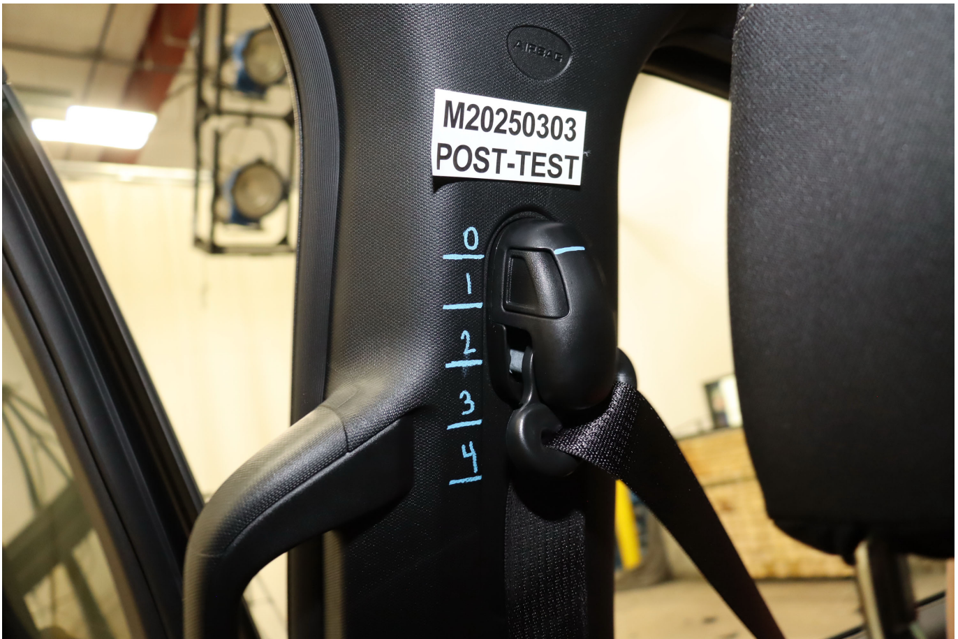
Photo No. 039 - Post-Test View of Belt Anchorage for Driver Dummy
